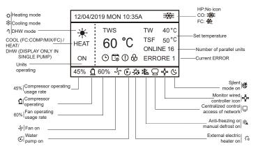
Set temperature; TWS/T5S:SETTING TEMPERATURE; TW:TOTAL OUTLET WATER TEMPERATURE, T5:TANK TEMPERATURE; TSF:SAFE TEMPERATURE;
